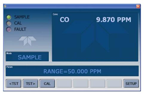
Figure 3-2: **Display Screen and Touch Control**
